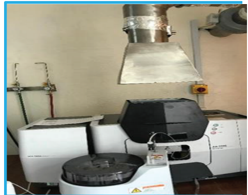
Fig.12. Installed Atomic Absorption Spectrophotometer Equipmen
