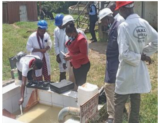
In - situ water quality measurement and sampling- Final effluent
