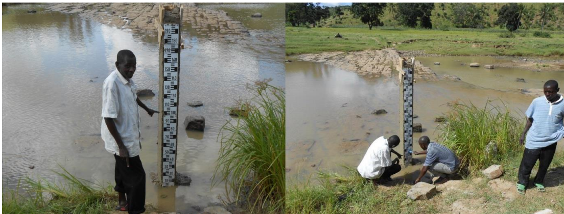
Figure 3.4: Concrete post installed at Mwache 3 MB02 and Gauge reader being trained reading in Athi Catchment.
