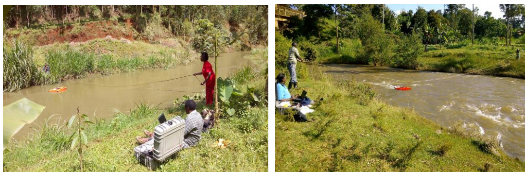
Figure 3.5: Flood flow monitoring by use of ADCP at Chania 4CA03 and Gura 4 AD01 in Tana Catchment
