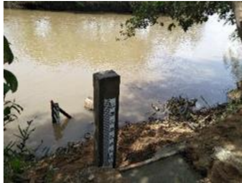
Figure 3.3: Rehabilitated RGSs 1AD02 Malakisi (left) and 1DA01 Nzoia at Webuye (right)
