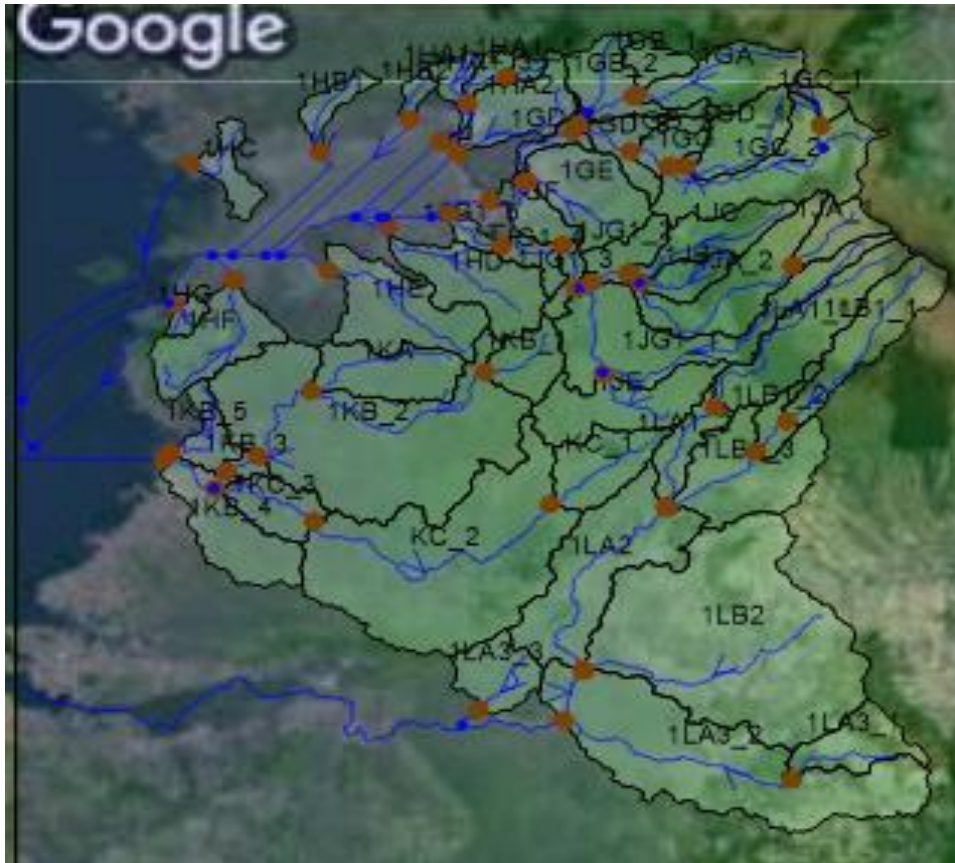
Figure A3-31: Lake Victoria South Basin Natural model configuration in MIKE HYDRO Basin
